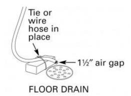
The photo below is an example of an air gap at the floor drain. Even if the floor drain were to back up with sewer water, the water wouldn't come in contact with the end of the discharge hose. Also, note that the cover for the floor drain has been cut out a little bit; if this wasn't done, the discharge from the water softener would probably splash water all over the place.
